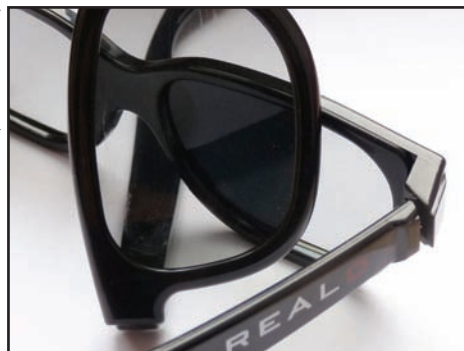
Figure 4 – Two pairs of RealD glasses are juxtaposed to demonstrate the alternate polarization of the lenses. Films digitally projected in theaters using the RealD circular polarization method display alternate digital frames for left and right eye at 144 frames per second.
